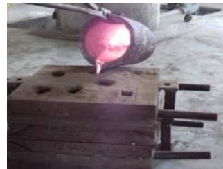
Fig 5: Molten metal poured into the sand mould
